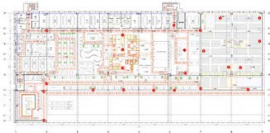
Figure 2 - Schematic of the room and location of sensors measuring indicators of fire hazards
